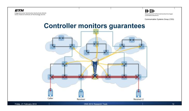
• After establishing the path, the controller continues to monitor the performance of the path via instrumentation at the data plane anchor and possibly at the endpoints.
