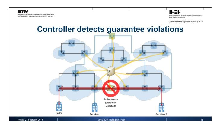
• The controller can detect violations of QoS guarantees, or even a completely failed link.
